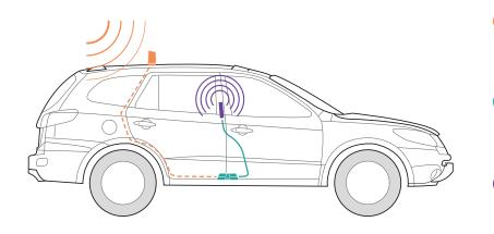
**Receives signal:** The powerful antenna reaches out to access voice and data signals, then delivers them to the booster.
